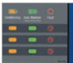
Battery fault detection LEDs
